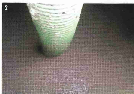
A Doda wet system Bio Separator (1) installed at A1 Organics in Denver depackages incoming organics into a slurry (2) consisting of about 10 percent solids, which gets mixed with bulking agents (3) for composting in windrows.
