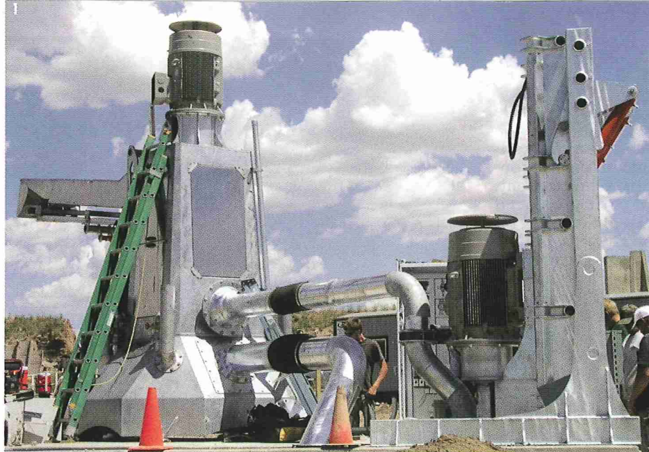
A Doda wet system Bio Separator (1) installed at A1 Organics in Denver depackages incoming organics into a slurry (2) consisting of about 10 percent solids, which gets mixed with bulking agents (3) for composting in windrows.
